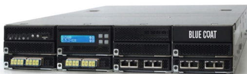
Figure 3-6: Sample SSL visibility appliance from Blue Coat.
