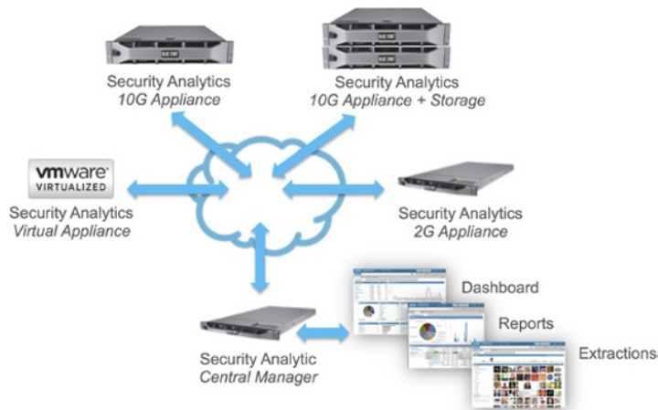
Figure 3-5: Distributed security analytics architecture.
